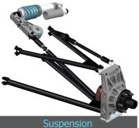
Double-wishbones meet inboard dampers and adjustable anti-roll bars front and rear.
